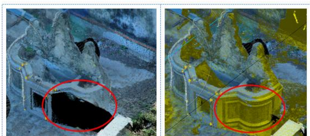
Figure 4 The 3D point cloud mode of the foreyard of this building scanned by Ground Lidar (left); the 3D point cloud mode after combination (right)
