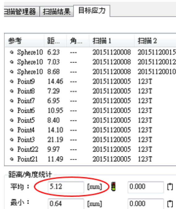
Figure 5 The Combined Error of 3D Point Cloud Modes Got from Ground Lidar and SfM(by FARO SCENE)
