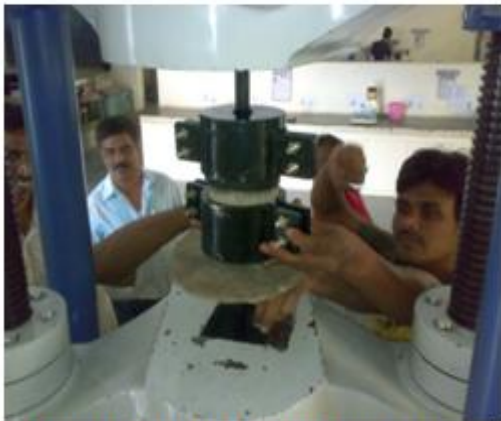
Photograph 5.2 Direct Tensile Test
