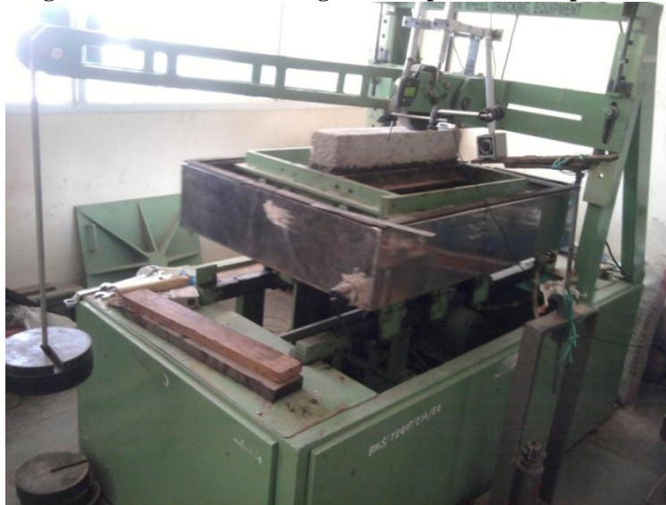
Photograph 5.4 Modified Immersion Wheel Trafficking Test Setup with Specimen
