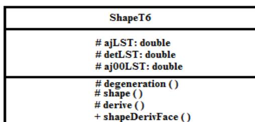
Figure 3.4: UML diagram for ShapeT6 with its attributes and operations
