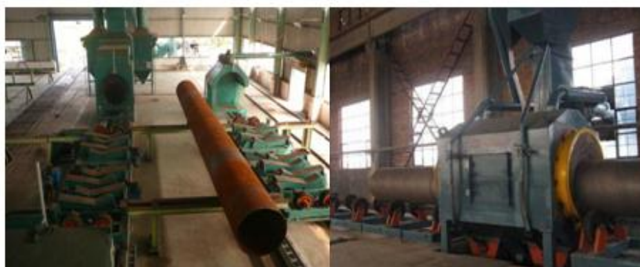
Fig5. Shot blasting Rust removal
