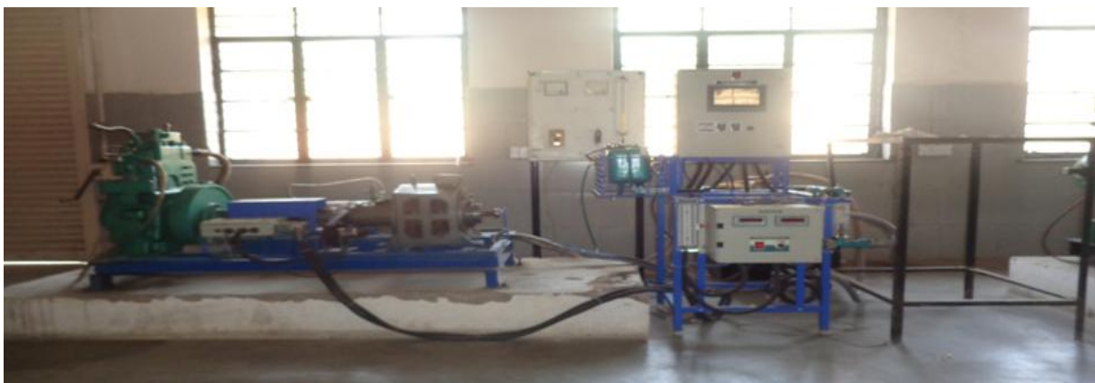
Figure.1 Computerized VCR Diesel engine test rig
