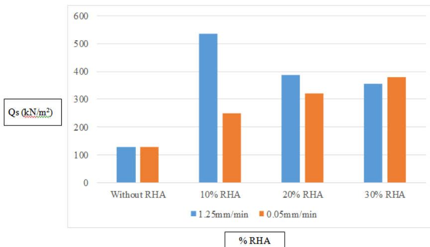
Fig. 9: Comparison of Safe Bearing Capacity for 1.25 mm/min and 0.05mm/min Strain rate
