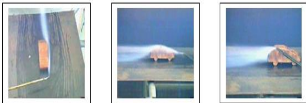
Figure (7) Flow visualization around Hyundai model
