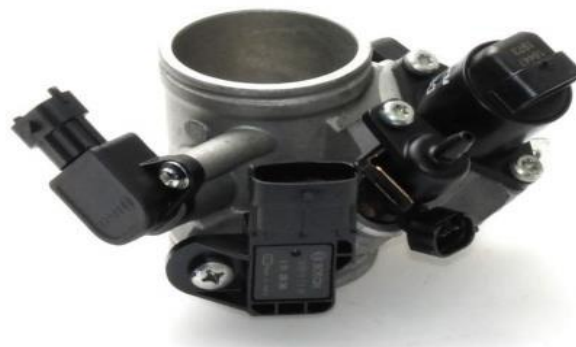
Fig.2 Throttle Body of KTM Duke 390
