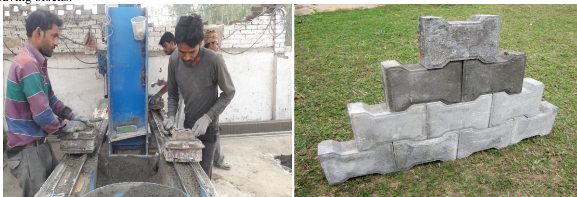
(a) (b) Fig. 1 (a-b): Photographs of fabrication of road paving blocks
