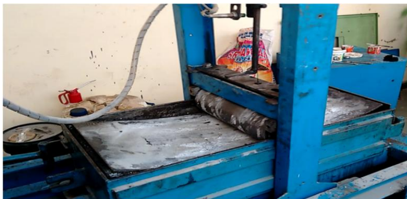
Figure 1: roller compactor cum rut analyzer (RCRA)
