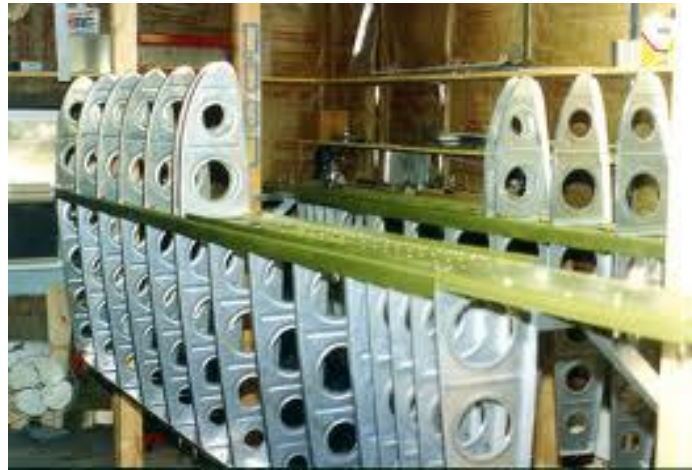
Fig. 5 Arrangements of ribs
