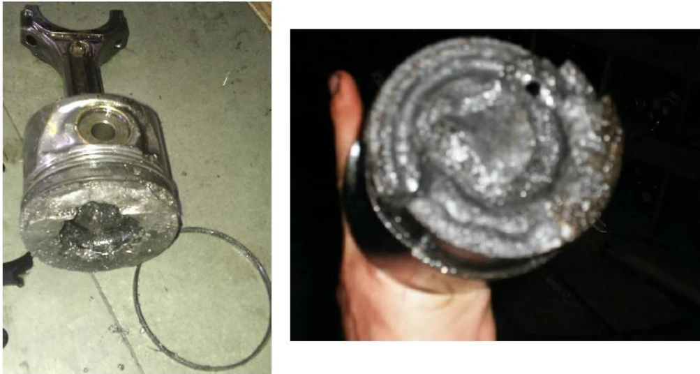
Fig. 2: Severe overheat failure of engine piston [4].
