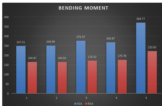
Figure 10:- Bending Moment comparison for G+12 Multi-Storey Building
