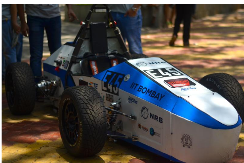
Fig.10. CF suspension linkages assembled with FSAE race car
