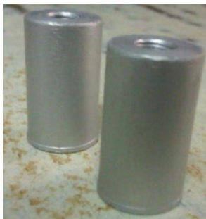
Fig.3. Aluminium inserts after anodized
