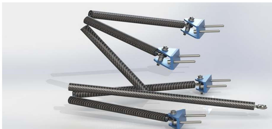
Fig.1. 3D model of the CFRP suspension linkages
