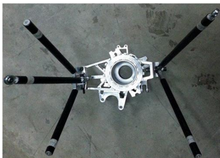
Fig.9. Assembled CF suspension linkages system
