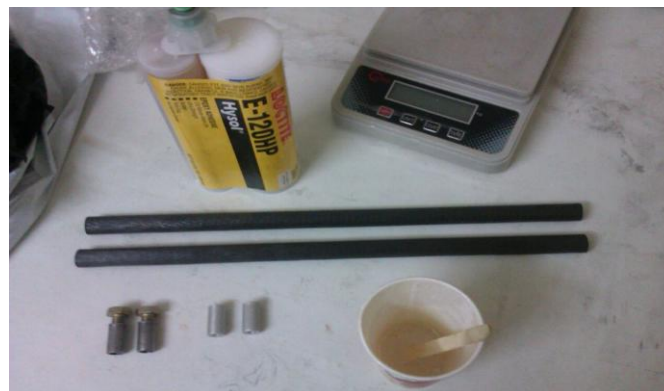
Fig.6. Bonding of CF rods with MS and Al inserts
