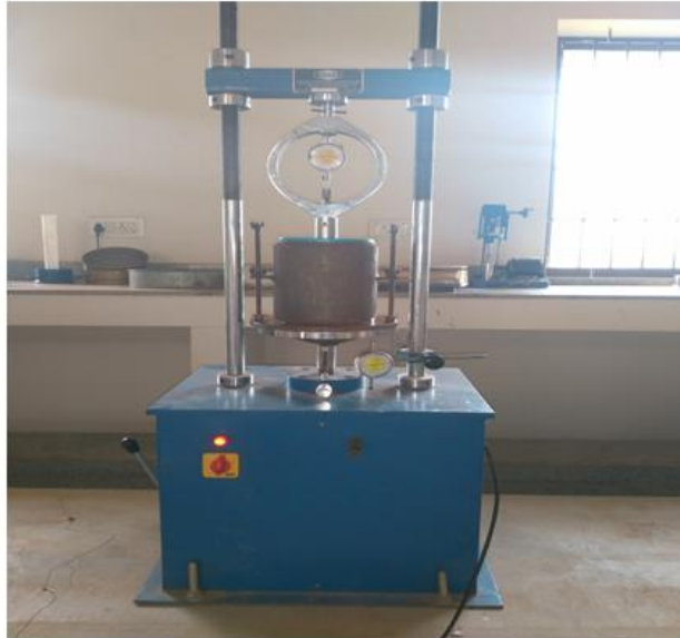
Fig 7: CBR testing machine
