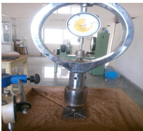
Fig 5: Square footing Test Setup
