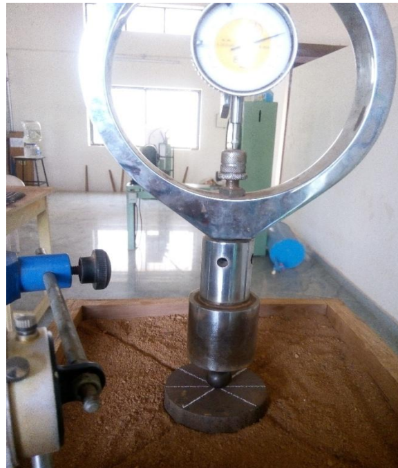
Fig 6: Circular footing Test Setup
