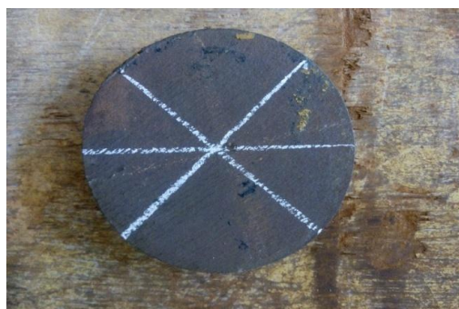
Fig 3: Model Circular footing
