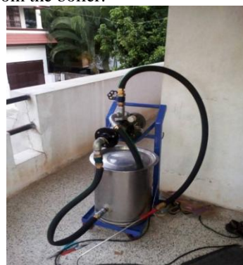
Fig. 13: Assembly of chimney cleaning system
