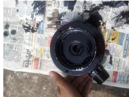
Fig. 9 Fabricated delivery section
