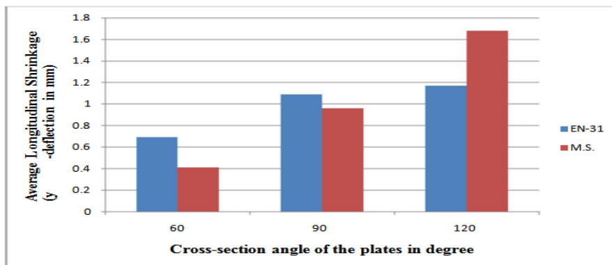
Graph 5.22 Graph of Average longitudinal shrinkage of 4mm.thickness plate of EN-31 and M.S
