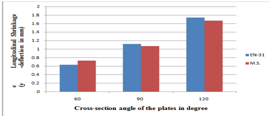
Graph 5.23 Graph of Average longitudinal shrinkage of 5mm.thickness plate of EN-31 and M.S
