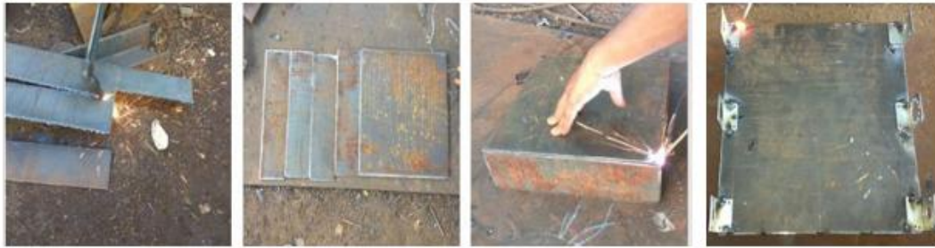
Fig. 6: shows the manufacturing of robot body frame.
