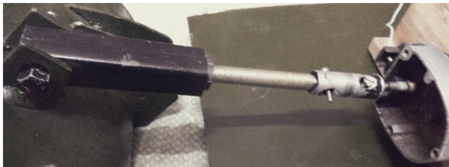
Fig. 7: shows the fabricated linear actuator
