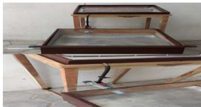
Fig: 5 Solar Still with Power Generation
