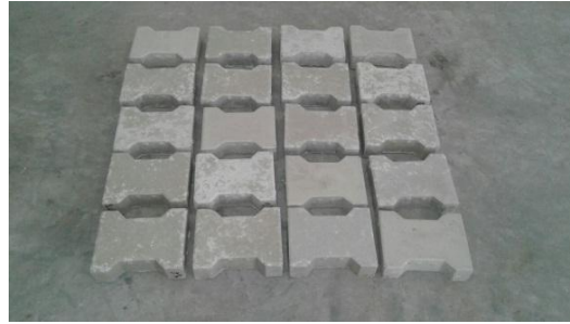
Fig.2. Paver blocks ready for test
