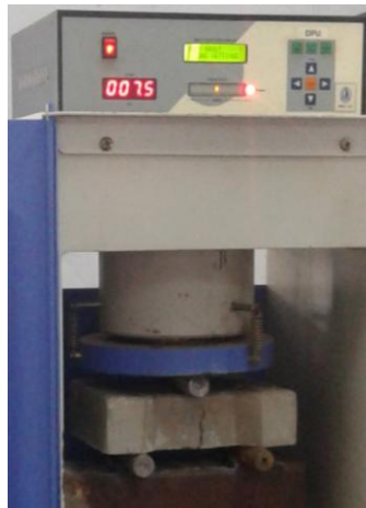
Fig.4. Test set up for flexural strength
