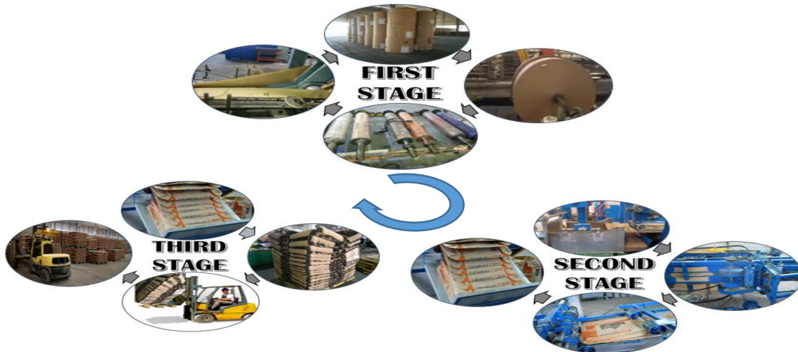
Fig. 2: Manufacturing processes of cement bags
