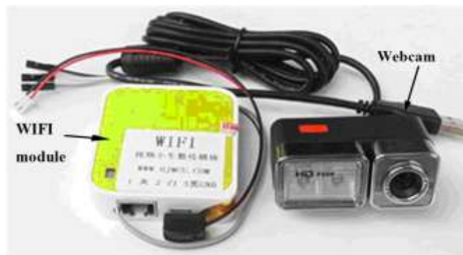
Fig.2 Webcam and WIFI data transmission module of the greeting robot
