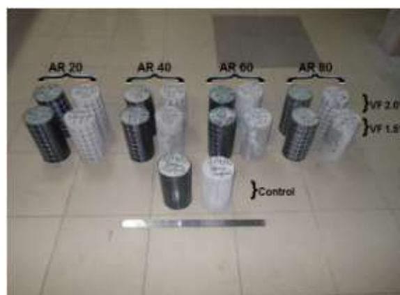
Fig. 2. Confined and Unconfined Concrete Cylinders
