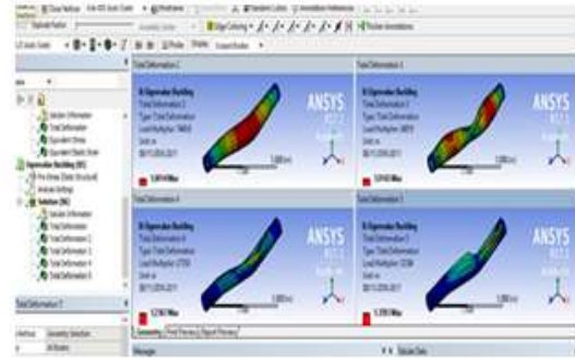
Figure 4: Buckling mode shape for Schedule 40
