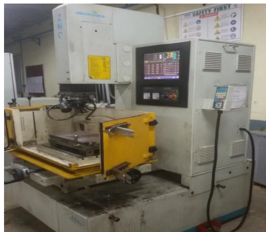
Fig. 2.1 Pictorial View of Electrapuls PS 50 ZNC electrical discharge machine
