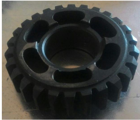
Figure 5: Existing (Baseline) Third Gear
