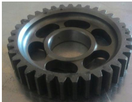
Figure 3: Existing (Baseline) First Gear
