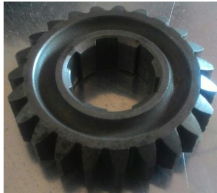
Figure 6: Existing (Baseline) Fourth Gear
