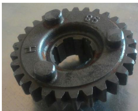
Figure 4: Existing (Baseline) Second Gear
