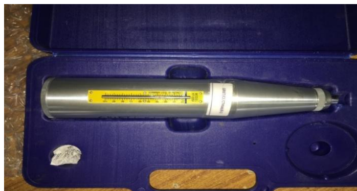
Figure 4: Rebound hammer used
