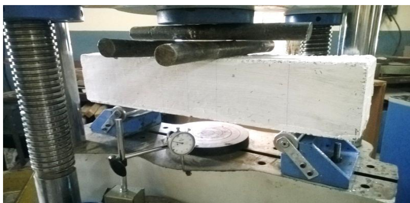
Figure 9: Experimental Setup of Four Point Load Test
