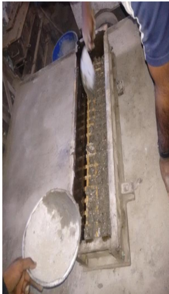
Figure 7: Bamboo-strip-mat Arrangement in Beam (3 mat)
