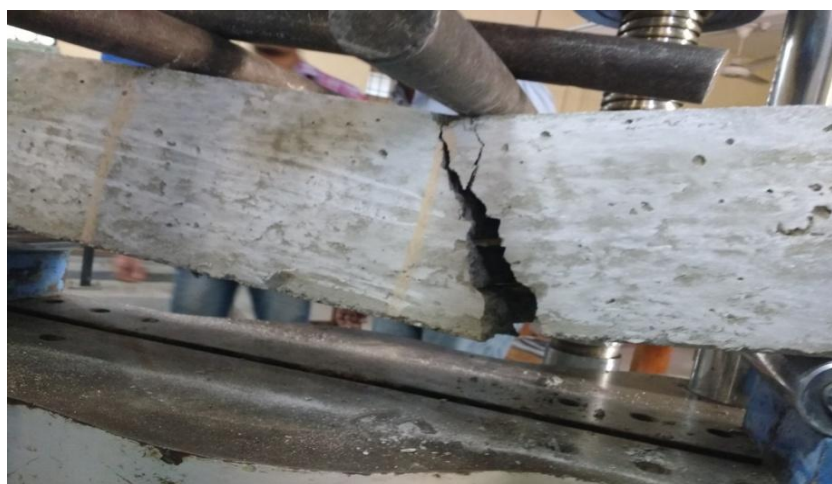
Figure 18: Four Point Loading Test on 3 Bamboo-strip-mat Concrete Beam
