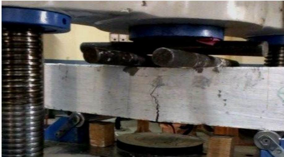
Figure 15: Four Point Loading Test on 1 Bamboo-strip-mat Concrete Beam
