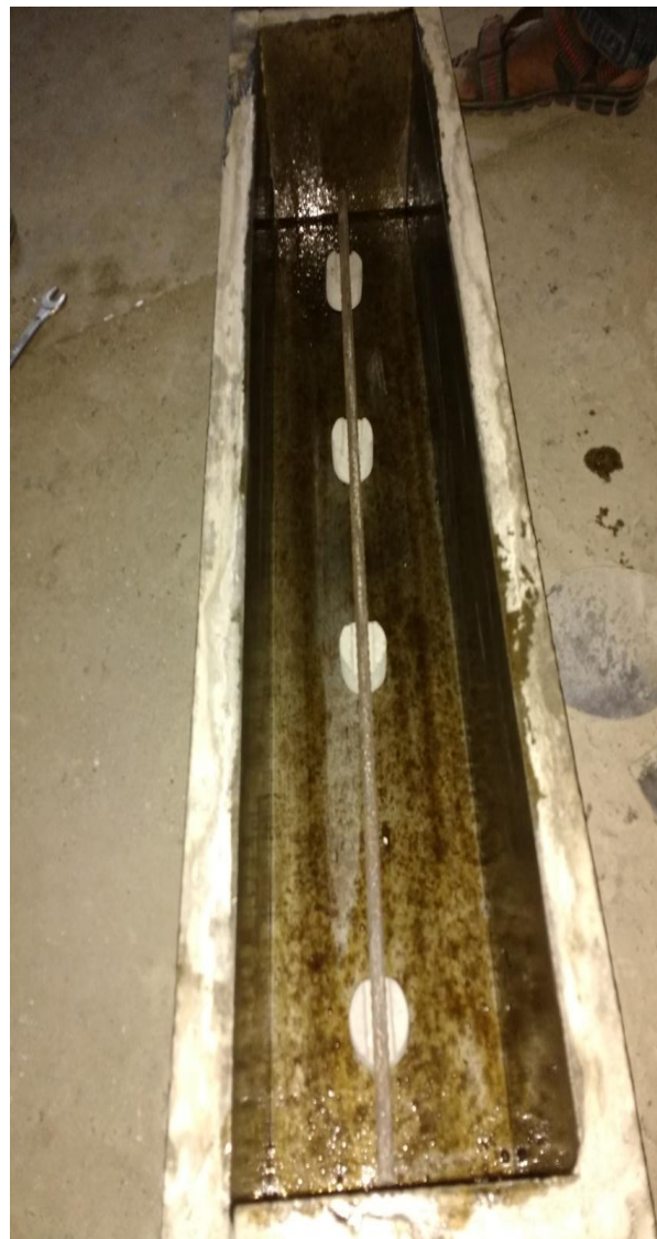
Figure 4: Arrangement of one TMT steel bar in Beam mould
