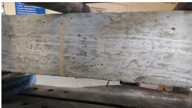
Figure 10: Placing Specimen for Four Point Loading Test
