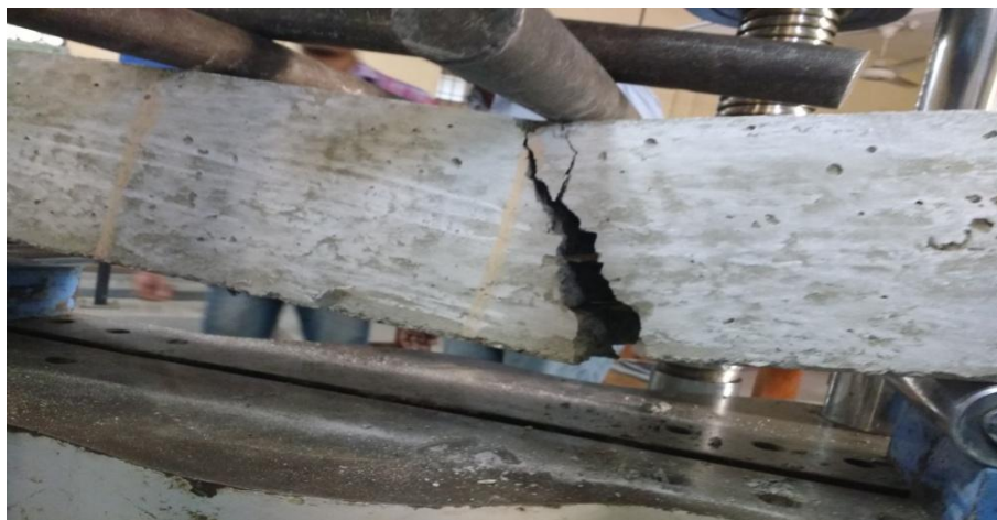
Figure 16: Four Point Loading Test on 2 Bamboo-strip-mat Concrete Beam (1)
