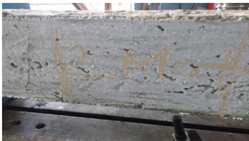
Figure 17: Four Point Loading Test on 2 Bamboo-strip-mat Concrete Beam (2)
