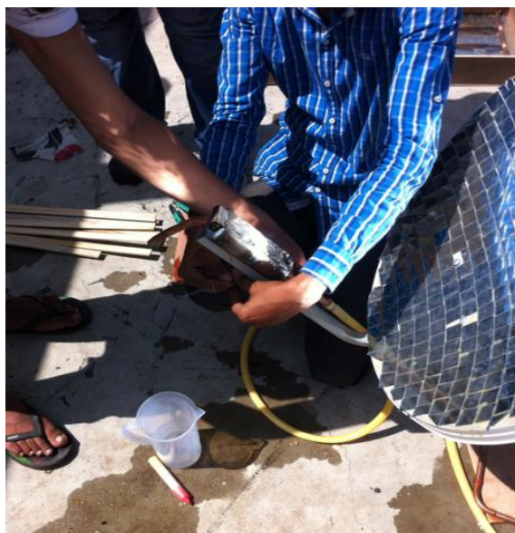
Fig 9 Setting of Wax box at Focal Point
