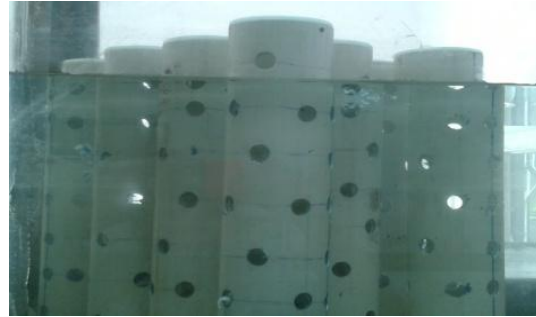
Figure (3c) Piles breakwater models
