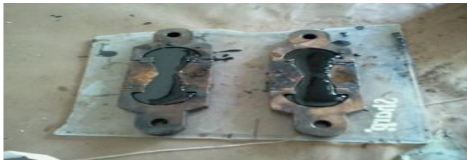
.Molds for Ductility Test
