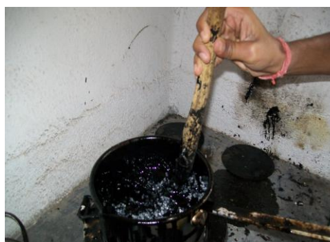
Mixing of EVA in Bitumen
