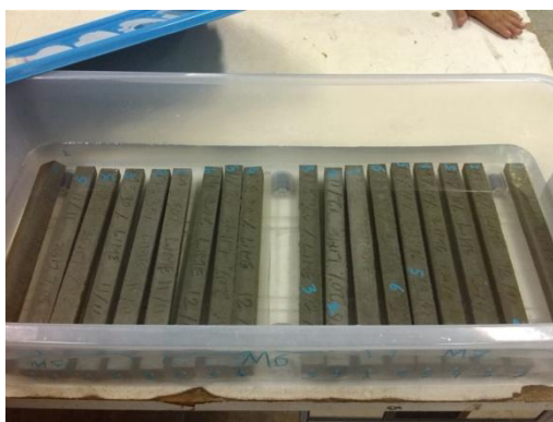
Figure 2: Mortar bars immersed in Na 2 SO 4 solution
