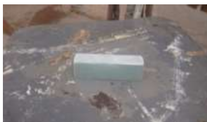
Fig shows block made of silica powder and GP resin
