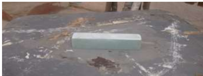
Fig shows block made up of silica powder and GP resin
