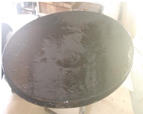
Fig 5.1: Applying of gel coat
