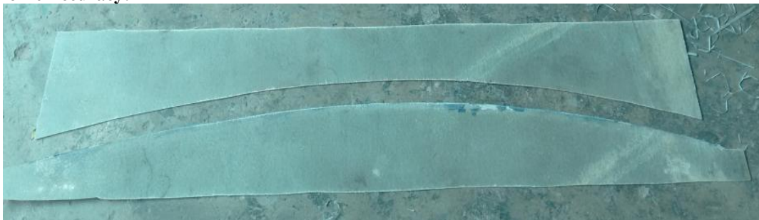
Fig 5.6 : Templet for Mould and Final Product
