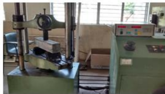
Figure 4 Testing of Prism Specimen
