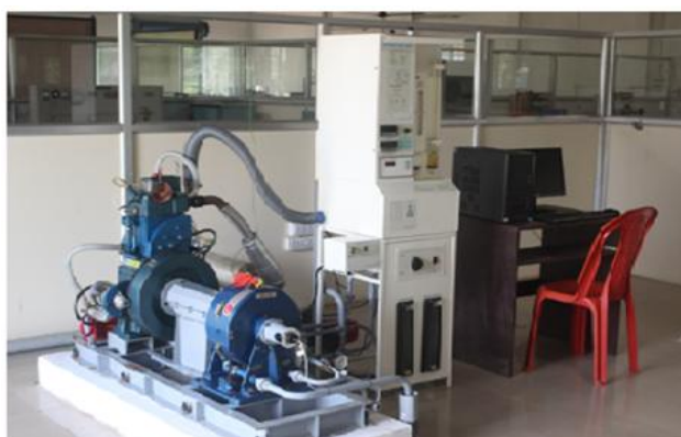
Fig. 6 Variable compression ratio test rig
