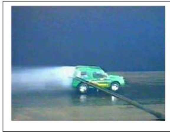
Figure (9): Re-circulating bubble or spiral vortices at the rear part of Pajero model
