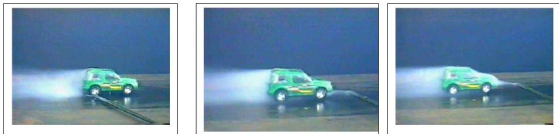
Figure (7): Flow visualization around Pajero model
