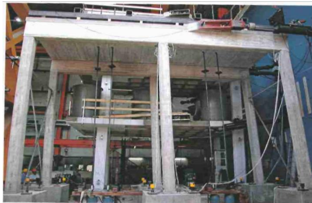
Fig. 4 Loading the practical frames.
