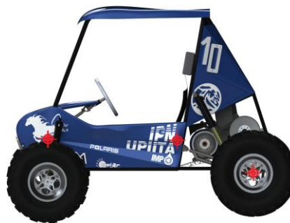
Fig. 7 Component of the program for the linear encoder. Fig. 8 Accelerometer location in the vehicle (red points).
