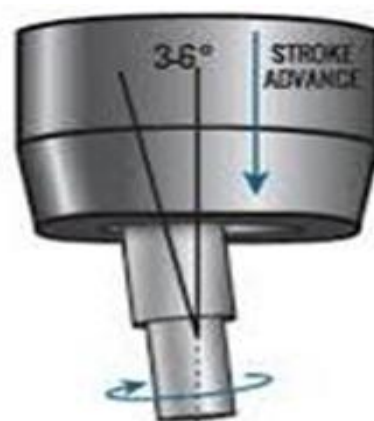
Figure 3 (iii): orbital forming setup
