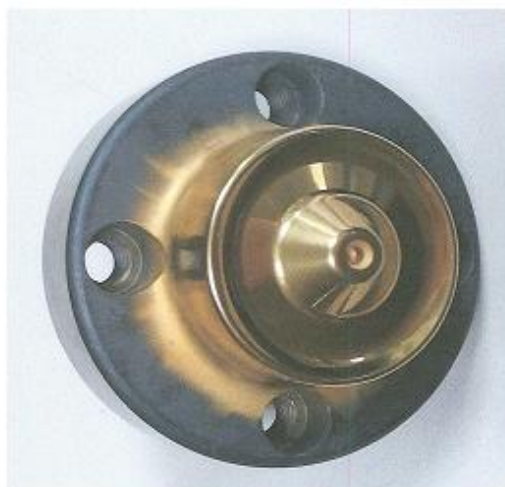
Figure 3 (ii): orbital forming Peen tool
