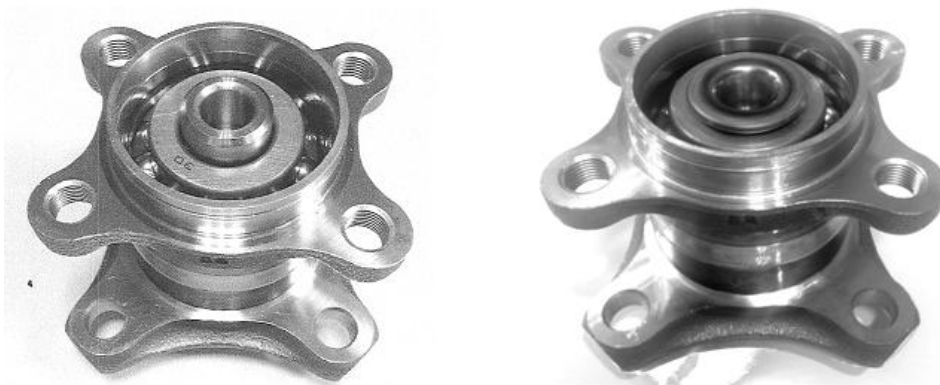
Figure 3 (v): Generation-3 bearing before and after orbital forming process
