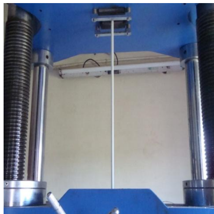
Fig. 3 GFRP reinforcement under Tension test
