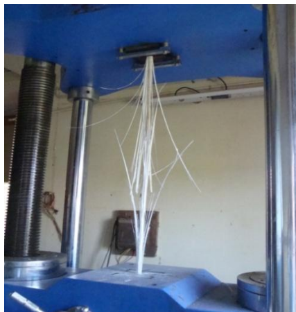
Fig. 4 Tensile Failure Mode of GFRP Reinforcement
