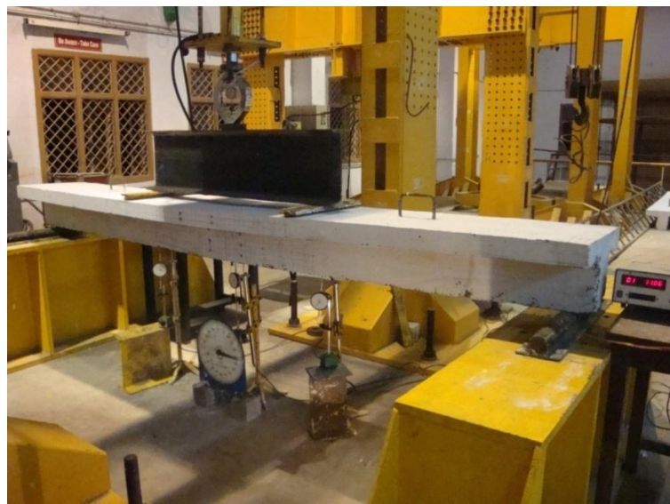
Fig.8 Flexure Test of Flanged Beams under Static Loading Condition
