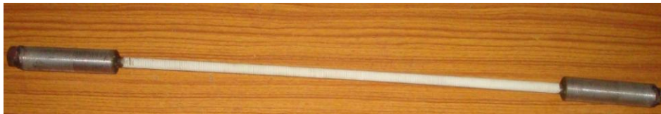
Fig. 2 GFRP Reinforcements with End Anchorages for Tensile Test
