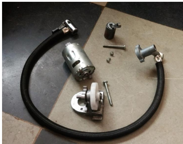
Fig 6: Disassembled piston-cylinder type air compressor during research.
