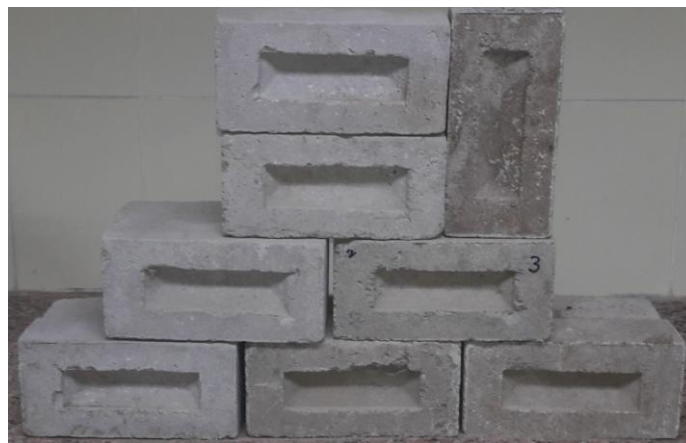
Fig. 3: Fabricated bricks using 100 % recycled fine aggregate
