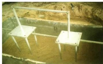
Figure 2.3: Model plane frame at base setup
