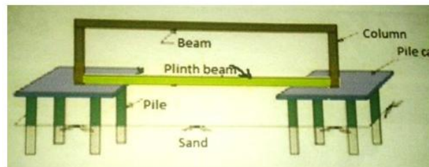
Figure 2.2: Model frame with plinth beam
