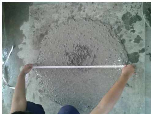
Fig 2.1.1 Check for slump flow
