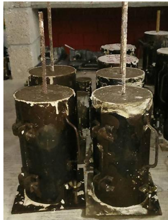
Figure 1.- Image of the poured earth cylinders used with a rod in the central part before demolding.
