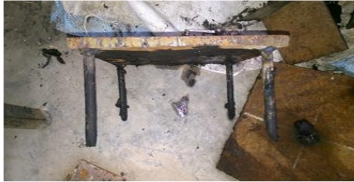
Fig.3: Model Pile Raft System
