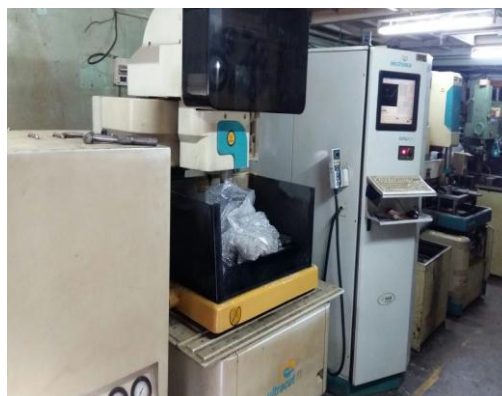
Fig. 1 Electronica Ultra cut WEDM set up
