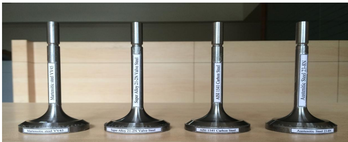
Fig 8. Components of exhaust valve (14mm fillet radius) to be tested
