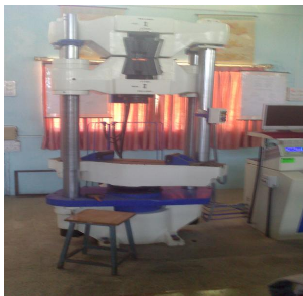
Fig 6. UTM set up for testing of exhaust valve
