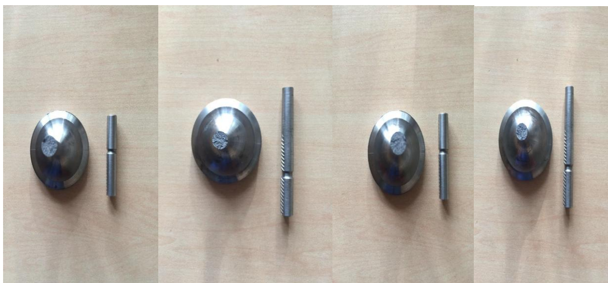
Fig 9. Tested component of Exhaust valve of 14mm fillet radius
