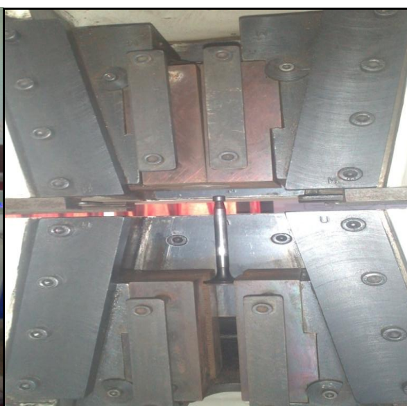
Fig 7. Exhaust valve testing fixture
